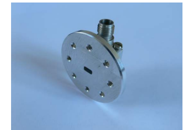
Custom Flanged 42 GHz (R500) Adapter
